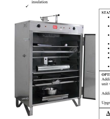
Constructed with 304 grade stainless steel, double walled with 16ga interior thickness/18ga exterior thickness with 2", 850 degree high temperature spin glass insulation for maximum heat retention.
