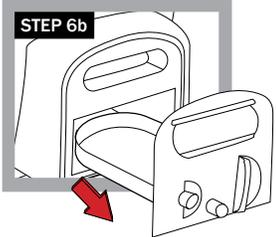
**WARNING: ALWAYS WAIT FOR ASH TO COOL BEFORE REMOVING ASH DRAWER. NEVER PULL OUT ASH DRAWER WHILE GRILL IS HOT.**
