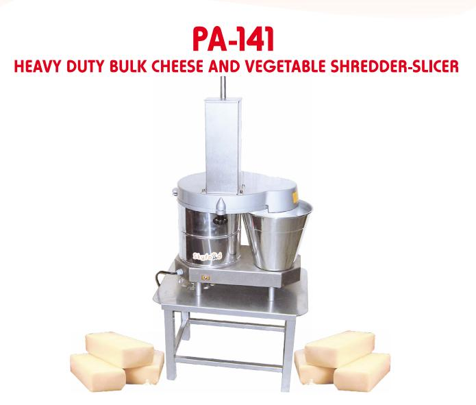
Slices, shreds and grates up to 880 lb per hour. This floor model Heavy Duty Cheese and Vegetable Shredder-Slicer features a large hopper that easily holds whole pieces of mozzarella and block type cheeses as well as vegetables. Powerful 1 1/2 HP motor guarantees power to oversized 17" shredding, slicing and grating discs. Oversized catch bucket allows continuous use. Heavy weighted pusher shreds cheese effortlessly. Easily comes apart for cleaning.
