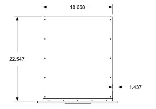
Dimensions shown are the actual physical dimensions. Additional clearances to the cabinetry are dependent on the tolerances of the cut-out. The suggested cut-out dimensions are listed in the chart below but these dimensions can be reduced if the tolerances are controlled. Please refer to the product manual for installation instructions.
