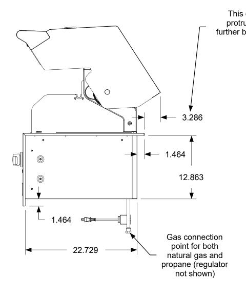
This dimension is the furthest point the dome protrudes back as it opens. It is 3.286 inches further back than the rear flange of the cabinet shell. 12.863 1.401 — 1.401 1.103 32.538 Distance to gas and electrical connection
