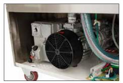
Powerful Vacuum Pump 3 HP oil rotary pump.
